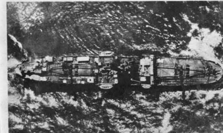
Merchant ship is designed for cargo capacity. Notice lack of taper, blunt bow and stern, constant beam throughout amidships section.
